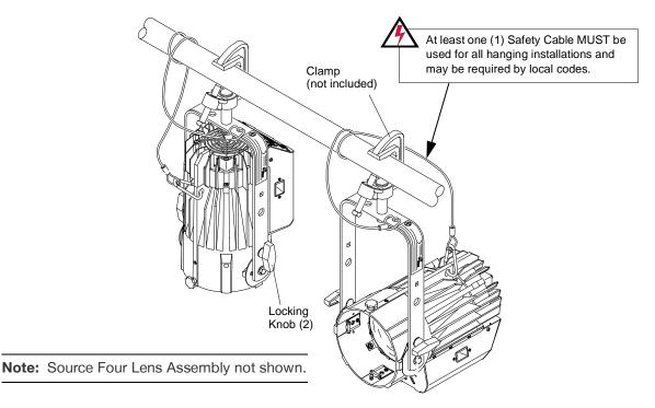
Figure 3: Standard Hanging Configuration
