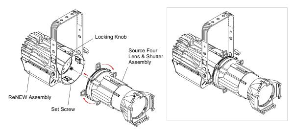
Figure 2: Attaching Source Four Lens Assembly
