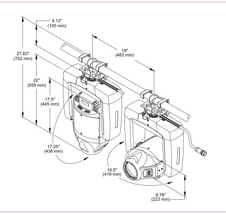
POSITIONING: Can be mounted in any orientation. SPACING: Hangs on 19 in. (483 mm) centers. WEIGHT: 29 lbs (13.2 kg)
