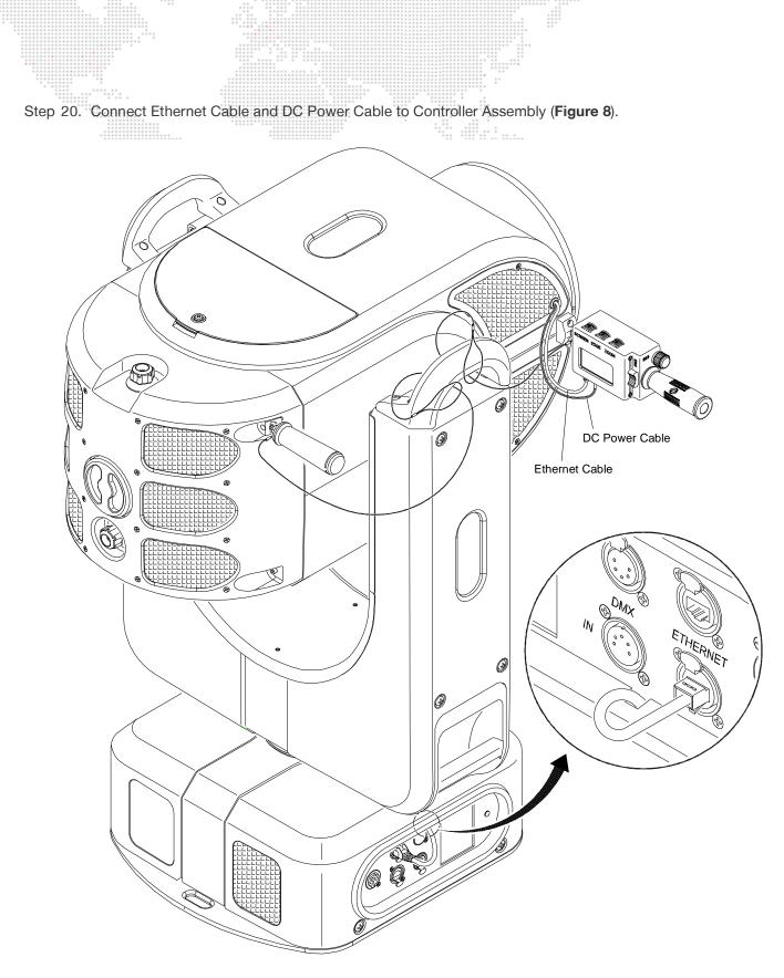
Figure 8: Connecting Power and Data Cables
