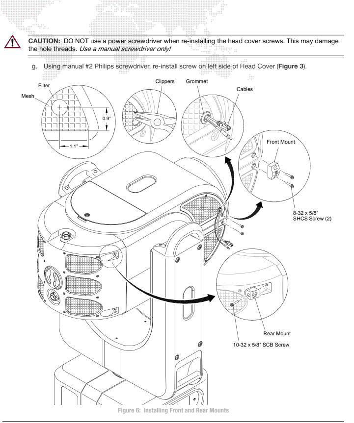
**Note:** The Rear Mount is used to connect the rear Handle. The Handle can be installed in one of two places. Refer to **Figure 7** for a view of both options.
