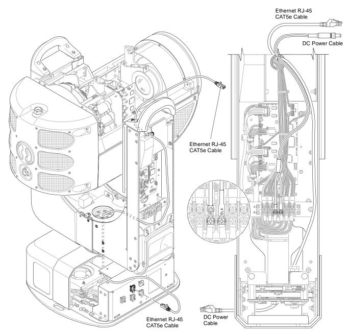
Figure 4: Installing Power and Data Cables
