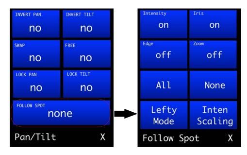
When any or all mechanisms are enabled for followspot control, "FSC Active" will be displayed in the **Comm** menu. The DMX channels associated with the active FSC mechanism(s) will be highlighted in yellow to indicate that those values come directly from the Followspot Controller and are not DMX-controlled.
