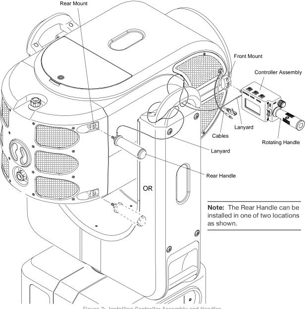
Figure 7: Installing Controller Assembly and Handles.
