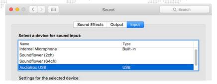
**CAUTION!** For TC Reader, the default audio input needs to be selected <u>before</u> the application is launched. If changes are made to the default input, then the TC Reader application will need to be quit and relaunched.
