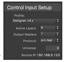
**CAUTION!** The Active Layers and Output Masters pop-ups will always show the maximum allowed quantities no matter which version of Mbox license is active. While this may make it seem like it's possible to have 24 layers with an Mbox Mini license, this is not the case! The usable layers and output masters will always be limited by the active license.
