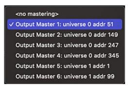
The output master assignment pop-up will show a list of the active output masters. The number of active output masters is set on the Patch tab (refer to "Patch Tab: Control Input Setup" on page 51), and the total number of available output masters is limited depending on the version of Mbox (Designer/Studio/Mini). Each output master has a patch universe and address that is pre-assigned and shown beside the output master's name in the list.
