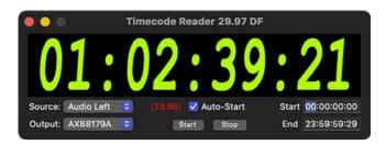
**CAUTION!** The TC Reader application is designed to perform best when receiving audio streams at a sampling rate of 44.1KHz. If a USB audio interface is being used to receive timecode on the computer, open the Audio MIDI Setup application on the computer and set the interface's sampling rate to 44.1KHz. If 44.1KHz is not available, choose the next lowest option.
