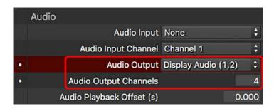
Clicking on the pop-up will reveal a list of available devices for output. The "OS Default" option will cause Mbox to use the audio output device that is selected in the System Preferences > Sound > Output pane. The "Built-in Output" option will cause Mbox to use the computer's built-in speakers. Selecting "None" will disable any audio output from the Mbox application. Other CoreAudio devices connected to the computer will be shown and can be selected.
