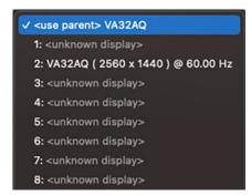
Clicking on the display pop-up for an output will show the list that includes all connected displays, and an option for "no display". In the case of sub-outputs, the "no display" option is replaced by the option: "<use parent>".
