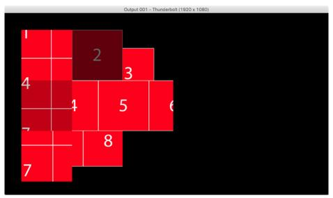
Through various changes to the opacity and texture X and Y values for each screen object it is possible to fade the screen objects in and out and to adjust which portion of the layer's texture appears on each of them:
