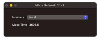
+ When using MboxTime from either a SMPTE source or the Mbox Network Clock application, it is possible to check that the Mbox application is receiving MboxTime by bringing up the [F9] HUD. The MboxTime value and type (Network or LTC) will be reported in the HUD:
