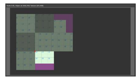
Note: In the image remapping preview area, the purple coloring is used to show a portion of the screen object that has no texture (i.e., where the screen object is fully transparent) due to the either the received control values or perhaps incorrect texture origin/width/height values for the screen object.
