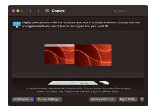
When connecting the video outputs of the Mbox server to a display device, confirm that the display device appears in the computer's System Preferences > Displays pref pane. On most Macs, the computer will automatically read the EDID of displays when they are first connected. It is possible to force the computer to reread EDID from connected displays by pressing the "Detect Devices" button on the Displays pref pane.
