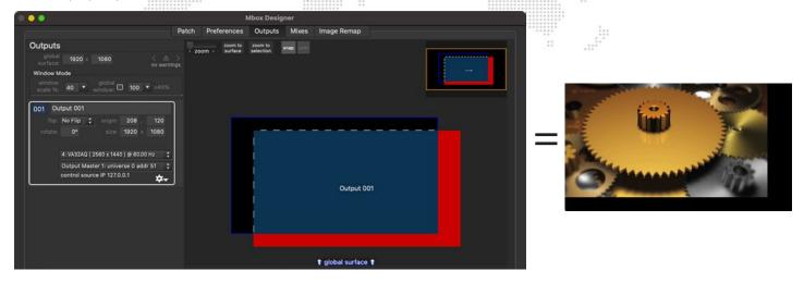
**Note:** Having a portion of an output outside the boundary of the Global Surface is not normal practice. If an output or mix extends outside the Global Surface's boundaries but needs to render content across its entirety, then either the output needs to be moved back so that all of it is on the Global Surface, or the Global Surface needs to be resized to fully enclose the output.
