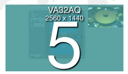
Clicking the Identify Displays button puts a temporary overlay onto each display connected to the computer. The overlays are colored and show the name, resolution, and unique index of the display. The name and number can then be referenced when assigning displays to outputs.
