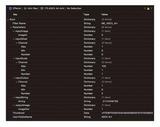
The root of the plist has been expanded to show the key:value pairs in the plist. Each key:value pair holds information critical to the operation of the effect, and both the key name and its value must be formatted correctly for the effect to work. To modify how an existing effect works, all that is required is to edit the appropriate values. Most values are simple numbers that describe a range for parameters of the effect, but they can get more complicated in some cases.
