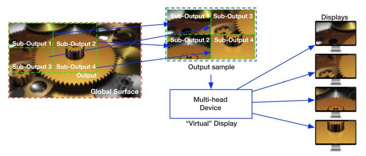
In this manner, imagery from anywhere on the Global Surface can be sampled and sent to the desired display device, whether that display is a single device or a multi-head device. Being able to move outputs on the Global Surface or sub-outputs on both the Global Surface and on their parent output is critical to getting the right pixels onto the display, as displays may want to have imagery that is unique, repeated, or even overlapping.
