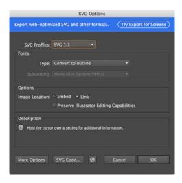
Step 11. After creating an digital gobo, changing the gobo's file extension from .svg to .svge will allow Mbox Daemon to generate thumbnails of the SVG file.
