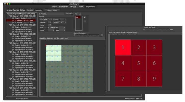
Step 19. With the configuration done, it's time to test it in Mbox. On Layer 1 - bring up the opacity, select the sample PNG as the texture on the layer, set the Image Remap parameter to a value of 001, and also supply the correct default external control data (for the opacity <u>and</u> texture X & Y position parameters) on Universe 16. The result should be something like this:
