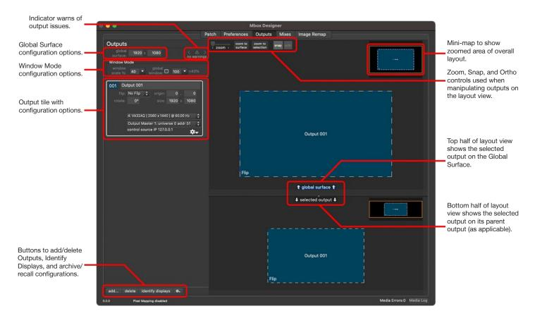
**Note:** Keystone and Warp for outputs are <u>not</u> configured on the Outputs tab. Keystone can be adjusted using Art-Net/sACN control from Director or a lighting console. Both keystone and warp can be pre-set using the Mbox Remote application. Refer to the Mbox Remote manual for more details.
