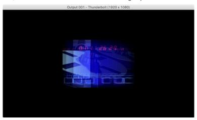
Step 5. To apply an effect to the layer, for example, set the Effect 1 parameter to a value of 6 (sepia tone) and set the Effect 1 Modifier A parameter to 255 (full). This should result in a sepia version of the same clip:
