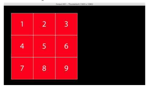
**Note:** Since the texture X & Y position controls default to 127, they will need to be set to that value to see the portion of the texture in the illustration to the left. With different values, the texture will move, and as it moves off the surface of a screen object, it becomes fully transparent.
