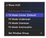
imagery will be scaled to fit a display that is a different size. There are four modes that control the fit – center (default), underscan, overscan, and anamorphic fit.
