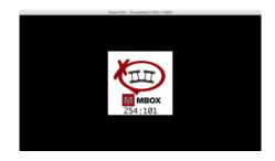
If the broken movie image appears or if poor playback is experienced, first confirm that the movie uses one of the Mbox preferred codecs. (Refer to "File Type Specifications" on page 39) If the movie is not using one of these codecs, it can be converted to a preferred codec using the AVF Batch Converter application. If the movie is already using the one of the preferred codecs, then the AVF Batch Converter application can be used in an attempt to eliminate the problem.
