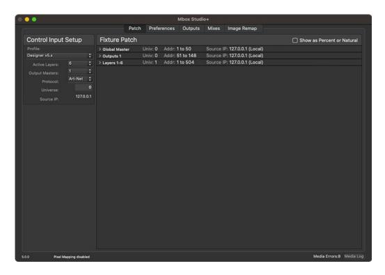
Upon launch, the Patch tab will be selected. This tab shows the server's mode, layer, and output configurations, plus its control protocol and universe. The Patch tab is used to configure control for the software and to view live parameter values. Refer to "Application Windows" on page 49 for more in-depth information about the Patch tab and the other tabs in the application.
