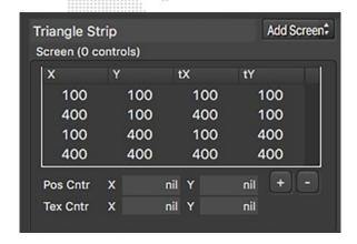
The four vertices are not ordered in a circular fashion around the perimeter the rectangle, but are ordered such that each set of three consecutive vertices describes a closed triangle. In the right-hand illustration above, the first, second, and third vertices create the one triangle, and the second, third, and fourth vertices create the other triangle. By their nature, the triangles share vertices - two in this case.
