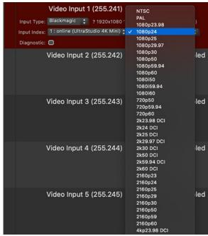
**CAUTION!** The choices on the input format pop-up may include formats that do not work with the connected video input device. Check the documentation for the input device to determine what formats it can receive. Do not select a format that the hardware does not support!
