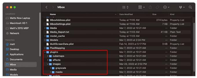
Within each of these folders, files will have 8-bit numbering. The Alpha Mask and Metalmage effects share the same folder, there may be up to 255 files, numbered 001 – 255 to share between those effects. The Custom Wipe Transition can only have up to 20 different input files – ten are used for hardedge wipes 001 – 010, and ten are used for soft-edge wipes 011 – 020. Numbering, naming, and file extensions conventions follow the same rules as standard Mbox content. [e.g. 001.MyFile.png]
