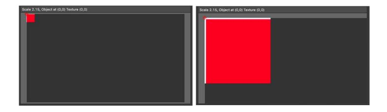
**Note:** All origins used in the image remapping editor are based on the top-left corner having coordinates of 0,0 - this related to the Mbox Global Surface, any outputs in Mbox, any screen objects, and any textures used.
