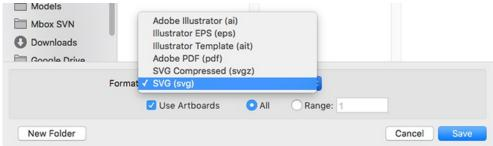
Step 10. Selecting the SVG file type will prompt a secondary pop-up window to set options when saving the file. When saving as an SVG file, the default values should be OK.
