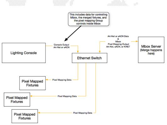
Figure 2: Example Merge Hardware I/O Diagram 2
