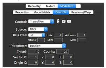
To add a control, click on the [+] button. To remove the currently selected control, click on the [-] button. If more than one control exists, use the up/down arrows or Control pop-up to toggle between the controls. Use the Source pop-up to select the type of control data being received - Constant, DMX (Art-Net or sACN), or SADI.
