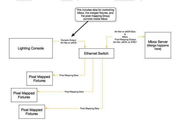
Figure 2: Example Merge Hardware I/O Diagram 2
