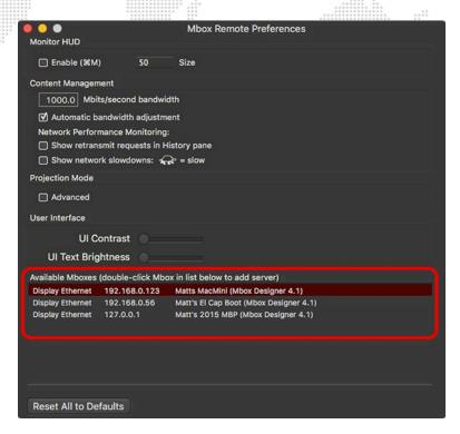
Step 3. When at least two servers have been added, click on the red button to close the preferences window. Managed servers are displayed as a scrollable list in the Servers column of Remote's main window.
