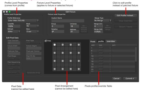
Pixel data is displayed in the window, but cannot be edited. However, it is possible to apply parked pixel overrides to existing pixels using the overrides tab. To add more parked pixels, use the Edit Profiles feature. Refer to <u>"Editing Fixture Profiles"</u> on page 104.
