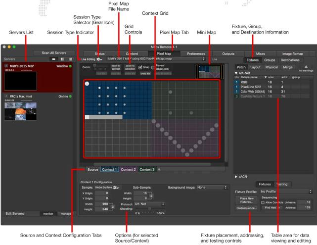
The grid area is the pixel mapping context. This is where fixtures can be arranged in order to assign their pixels to various areas of the screen image. The grid lines are colored white every tenth division. The fixture table to the right of the grid shows fixture patch and destination information. Fixtures can be selected on either the grid or in the table (they will become highlighted in both places). Other controls allow auto-addressing and testing fixtures.
