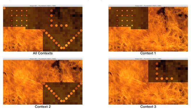
**CAUTION!** Showing the pixel mapping previsualization affects the video output of the Mbox application! If the same Mbox server is being used for both pixel mapping and video output, take care not to enable the pixel mapping previsualization when outputting video for the show.
