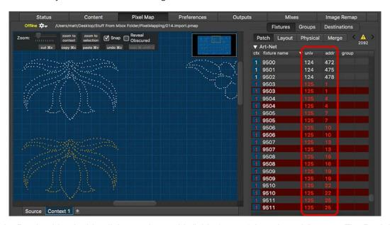
Step 4. In the Patch table, double-click on univ or addr field of one of the selected fixtures. The Re-Address Multiple Fixtures window will open.
