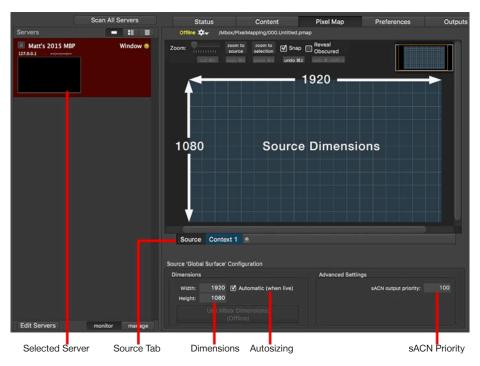
When a context is created and assigned to use a source, a tab for that source will appear. When a source tab is selected, the source's size (for the purposes of pixel mapping only) can be manually or automatically configured using the Source Dimensions controls in the lower portion of the Pixel Map tab.
