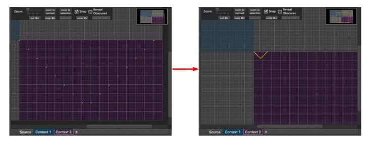
The context's sub-sample width and height can be changed by entering a math equation in the context's Sub-Sample fields. For example, '/10' (divide by 10) as shown below:
