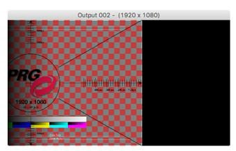
Step 6. At this point the outputs from Mbox would need to be connected to a pair of projectors to continue to adjust the vignette settings (including curve and gamma) to get the best blend results.
