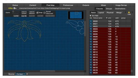
Step 3. Press [#P] to paste the fixture(s). They will be dropped where the cursor is located. The pasted fixtures will be automatically selected and addressing conflicts will be shown in the table.
