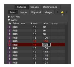
**Note:** To make changes to multiple fixtures at the same time, use the Re-Address Multiple Fixtures window. Refer to the instructions below.
