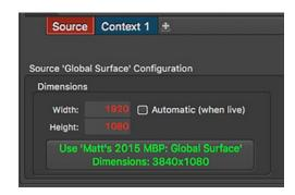
To automatically resize the source to match the new size of its rendering surface, press the button at the bottom of the Dimensions area.
