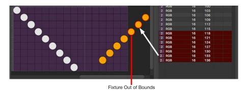
Geometry Tools can be used to adjust fixture placement. Refer to "Geometry Tools" on page 81.
