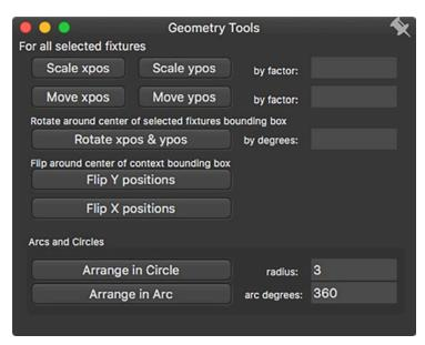
For example, when reducing the context size from 160 x 90 to 16 x 9, it would be time-intensive to manually move all the fixtures so they will fit into the smaller context. In this case, the Geometry Tools could be used to move all the fixtures at once. To do this, select all fixtures, enter a factor of 0.1 in the "by factor" field and click Scale xpos and Scale ypos buttons. (This will divide the scale by 10.) Once the fixtures are moved, then reduce the context size in the usual manner.
