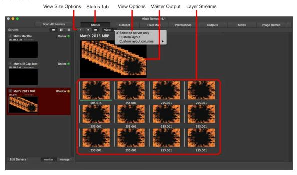
In the custom layout mode, server status can be setup by dragging a server into the status area.
