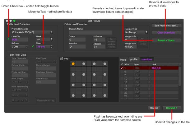
Fixture values that are edited to be different from the profile data are considered "overrides." Fixtures with overrides will have a magenta dot indicator in the Fixture table. If the Edit Fixture window is opened again these overrides can be cleared, thereby reverting to the original property from the fixture profile.
