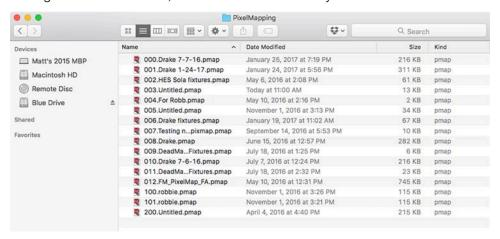
Like all 2D and 3D content for Mbox, pixel mapping files must be given an 8-bit numerical index as prefix to the file name. The index ensures that the files can be synced using the Content Management features, and also that they can be switched on the fly without reconfiguring the server or leaving Fullscreen mode (the switch can be made using Mbox Remote, Director, or a lighting console).
