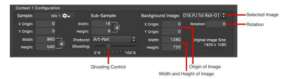
**Note:** When using Rotation, the background image is rotated around its X and Y origin rather than around its center. The X and Y origins may need to be set to negative numbers in order for the entire background image to be fully visible.
