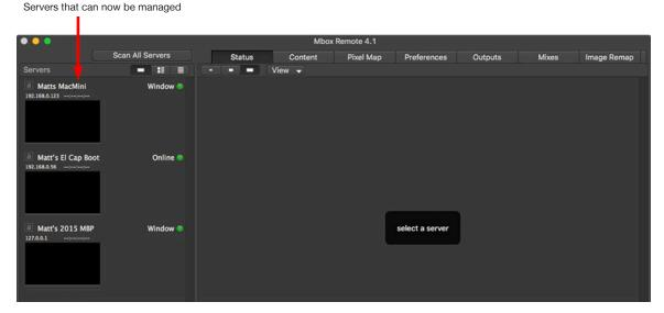
**Note:** No matter which tab is selected in Remote's main window, the Servers column on the left will always display the list of managed servers. The selected server in the Servers column will dictate what information is displayed or being edited on the selected tab.
