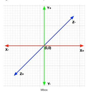
Most 3D modeling applications swap the Y and Z axes when compared to Mbox. The Y axis now being the towards <-> away and the Z axis being up <-> down. When exporting .obj files from your modeling application for use in Mbox, make sure to swap the appropriate axes to ensure the model appears with the correct orientation within the Mbox 3D environment.
