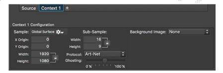
**Note:** Some text fields can perform math operations such as add, subtract, multiply, and divide. For example, if setting the Sample Width for a context to half of 1920, enter 1920/2 in the field then press [return] on the keyboard.
