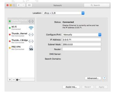
broadcast address. But in cases where the computer is connected to ArtPOLL compliant devices (e.g., Artistic Licence Ether- Lynx) Mbox can unicast universes to the specific IP Address for those devices. Note: If two more devices respond to an ArtPOLL replying that they require a universe of data, that universe will be broadcast instead of being unicast.
