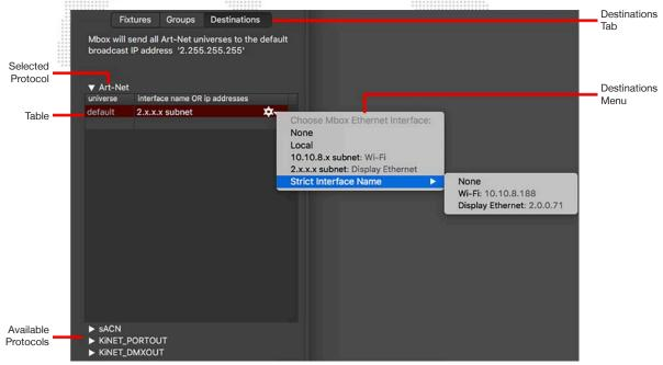
There is a separate area of the Destinations tab for each of the protocols. When the Destination tab is selected, the protocol of the current context will be displayed. A different protocol can be viewed by clicking on the name of the protocol.
