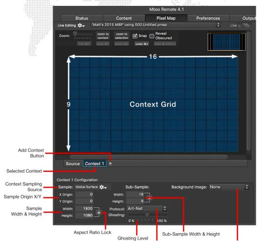
Contexts are configured using the Context controls in the lower portion of the Pixel Map tab.
