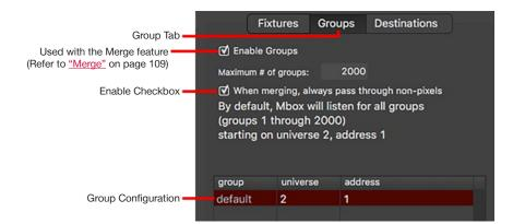
Mbox Remote allows up to 2000 Groups. If the default Group patch is used, all Groups will be patched sequentially starting with the start universe and address. Group controls will not be split across universes, allowing for a maximum of 102 Groups per universe (510 channels). Each group uses five 8-bit channels for control of Mode, Intensity Master, Red/Cyan, Green/Magenta, and Blue/Yellow.
