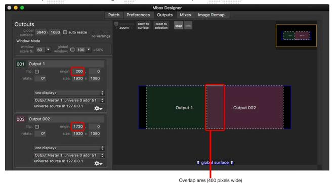
This will lead to the following result on the outputs from Mbox, note the repeated pixels caused by the overlap of the two outputs on the Global Surface:
