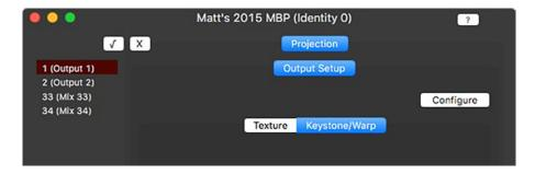
**Important!** To view the results of keystone/warp configuration created in Mbox Remote on an output, the output must either have no output master assigned, or must have the Output Master > Keystone Mode/Curve parameter set to a value of 0.
