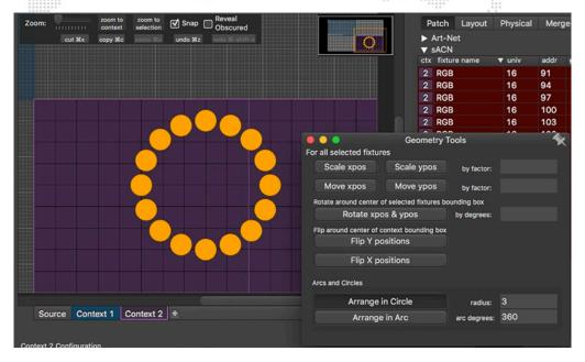
+ Arrange in Arc places the first fixture at 0 degrees and the last fixture at 360. The first and last fixture are placed on top of each other.
