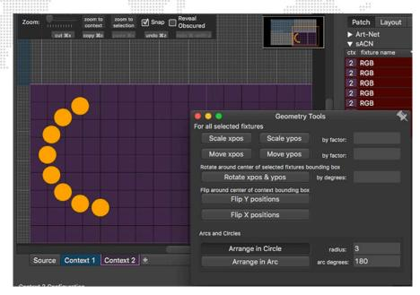
+ Arrange in Arc places the first fixture at 0 degrees and the last fixture at 180.
