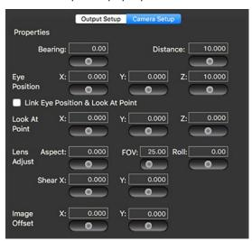
The camera's Eye Position and Look At coordinate are entered in generic real-world units (e.g. inches, feet, millimeters, meters, etc.). The system of units <u>must</u> be the same as the measurement units used when creating objects - either within a 3D modeling application or when making Topo objects in Mbox's Projection Editor window. (Refer to "Topography" on page 36)
