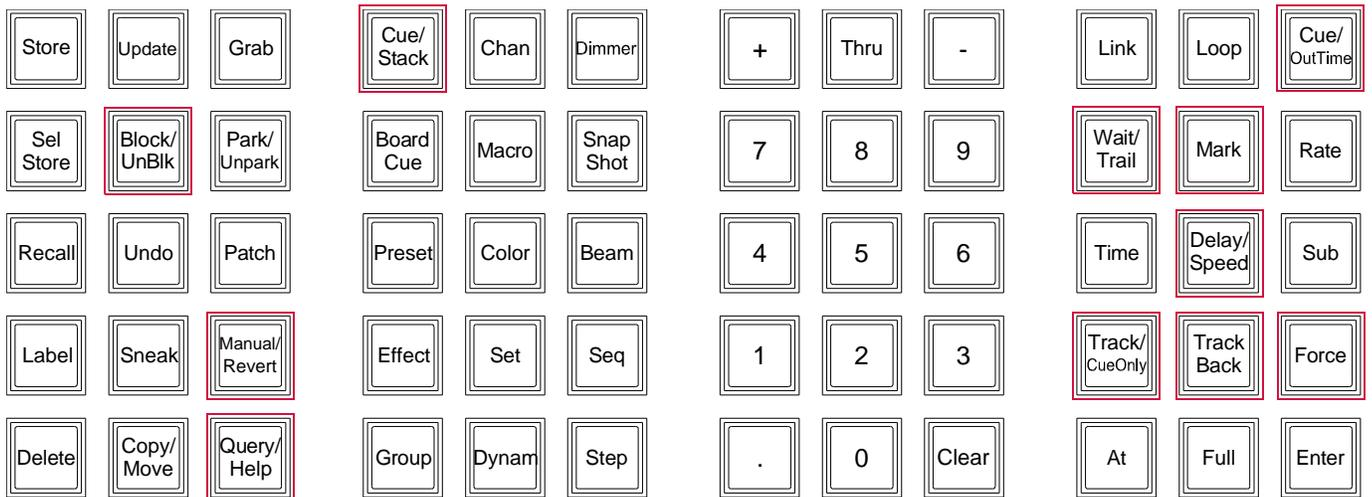
Figure 1: Updated Layout for V476/V676 Command-Line Keypad
