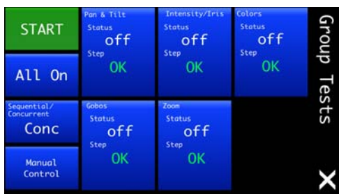
Group Tests Screen - Allows multiple luminaires to be tested when daisy-chained together.
