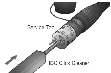
Figure 2-2: QUAD Service Tool Cleaning
