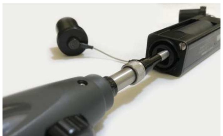
Figure 5-8: QUAD Coupler LC inspection
