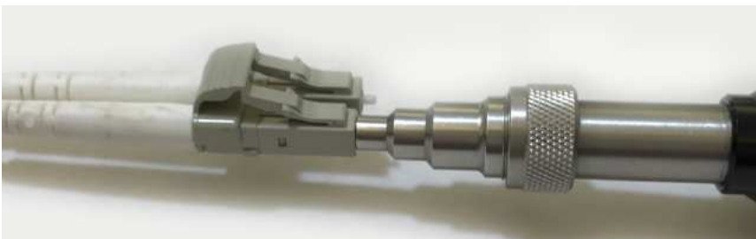
Figure 5-6: Installing the fiberscope on DUO LC fiber
