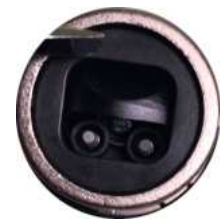
Figure 4-3: QUAD connector door partially opened
