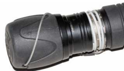
Figure 4-23: Proper Dust Cap cord orientation
