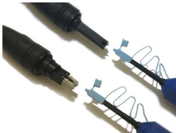
Figure 4-25: DUO (left) and QUAD (right) click clean detail without Service Tool
