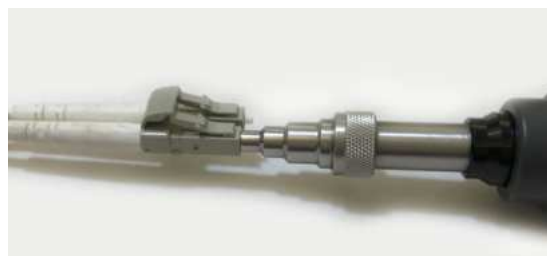
Figure 3-4: Inspecting LC ferrules
