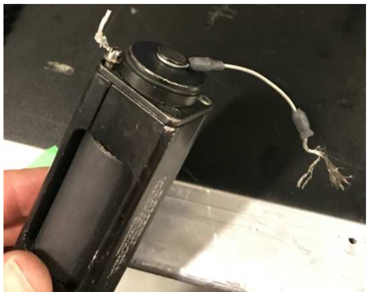
Figure 4-8: Coupler with destroyed cap cord
