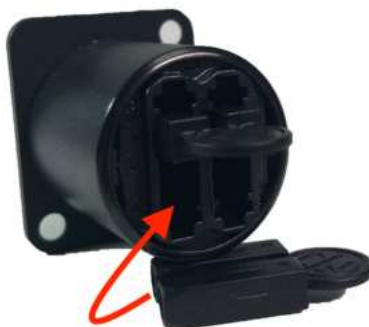
Figure 4-29: Installing rubber duplex seal
