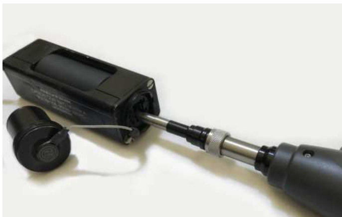
Figure 5-7: DUO Coupler LC inspection
