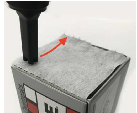
Figure 4-13: Cleaning fiber ferrules on QbE Box
