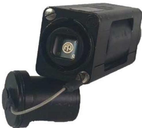
Figure 4-7: Coupler with good hardware
