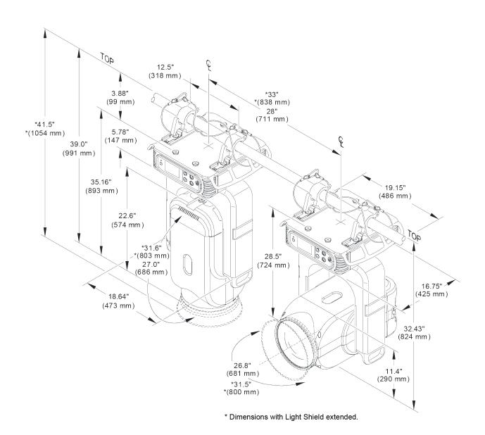
**POSITIONING:** Can be mounted in any orientation.
